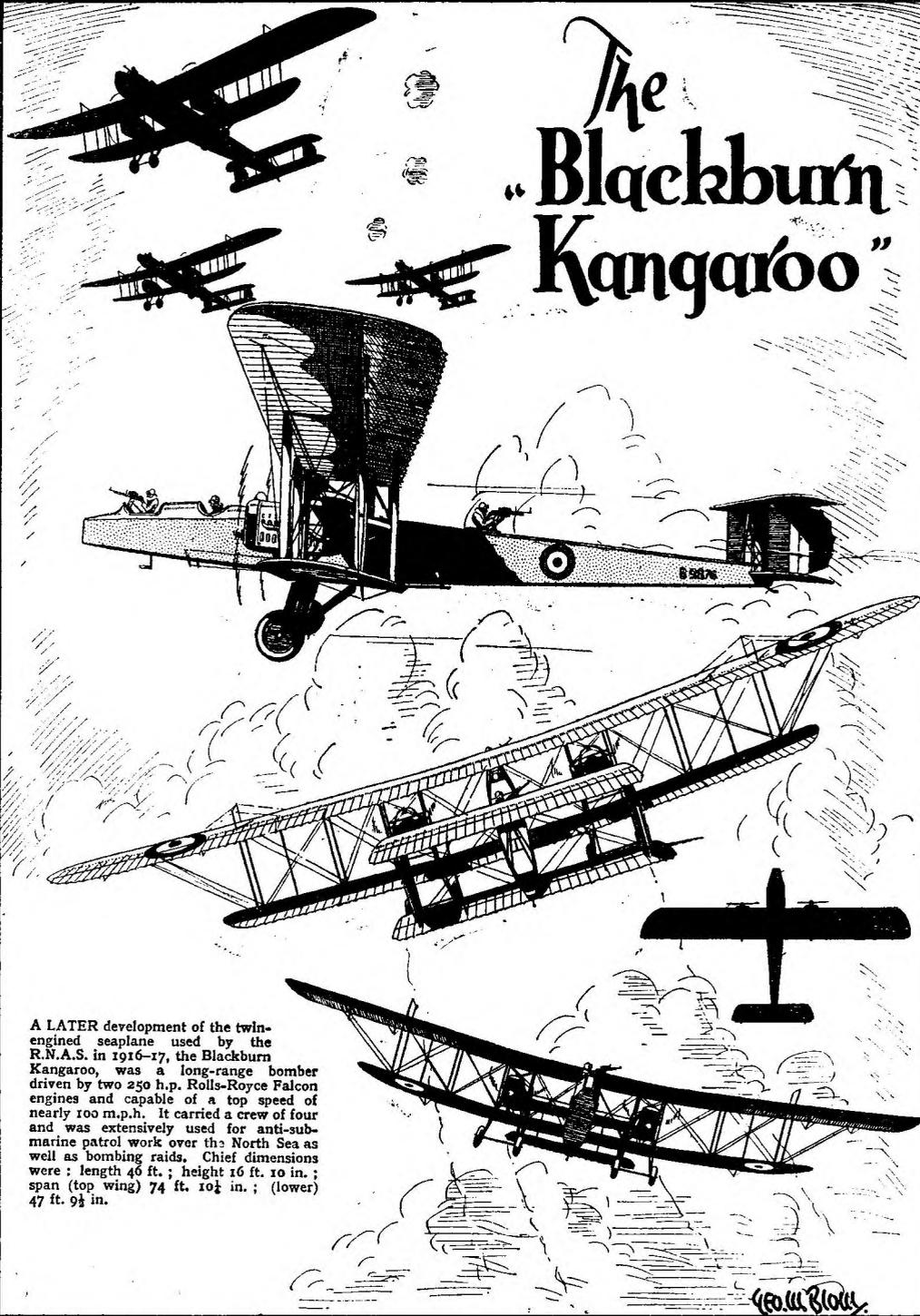
A LATER development of the twin-engined seaplane used by the R.N.A.S. in 1916-17, the Blackburn Kangaroo, was a long-range bomber driven by two 250 h.p. Rolls-Royce Falcon engines and capable of a top speed of nearly 100 m.p.h. It carried a crew of four and was extensively used for anti-submarine patrol work over the North Sea as well as bombing raids. Chief dimensions were: length 46 ft.; height 16 ft. 10 in.; span (top wing) 74 ft. 10½ in.; (lower) 47 ft. 9½ in.
